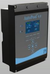
Process Pools (Pi's) MutoDrive<sup>®</sup> control sets the recirculation pump motor speed automatically based on residual biocide level. The biocide level is affected by biocide demand which is directly linked to the number of people using the pool or spa, therefore AutoPool<sup>®</sup> controllers can reduce pump speeds and electricity costs during periods of fewer bathers.
